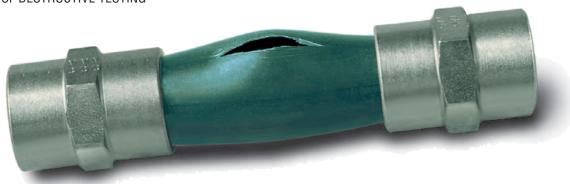
Destructive testing with 22x2 carbon steel tube The tube burst at 800 bars without any leakage or sweating from the sealing points.
