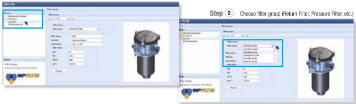
Choose filter type (MPF, MPT, etc.) in function of the max working pressure and the max flow rate  $\,$ Step (3)
