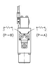
1) Note: The duty cycle refers to one coil only of each twin solenoid. The perm. duty cycle is only 50%, when both coils are energized simultaneously
