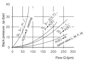
Input / consumer flow curve (Guideline, example directional spool valve with inflow controller type SL 5-52../..)
