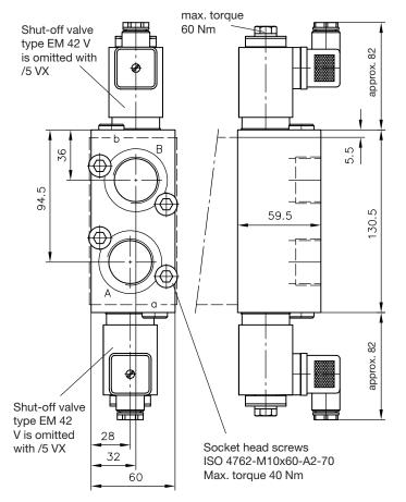
Pressure adjustment B-side with type /..AS.. BS A-side with type /..AN.. BN A-side with type /..AN..
