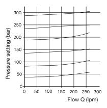
Secondary pressure limiting valves (Coding A., B.,; C., acc. to table 16 in sect. 3.2.1)
