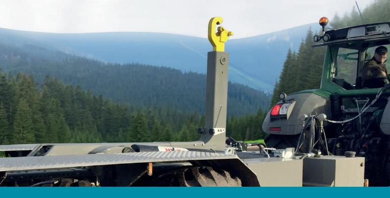
A fully automatic hydraulic drive system, the Copro-Drive System integrates tractor and machine drive systems into a single road train unit that copes with difficult terrain.
